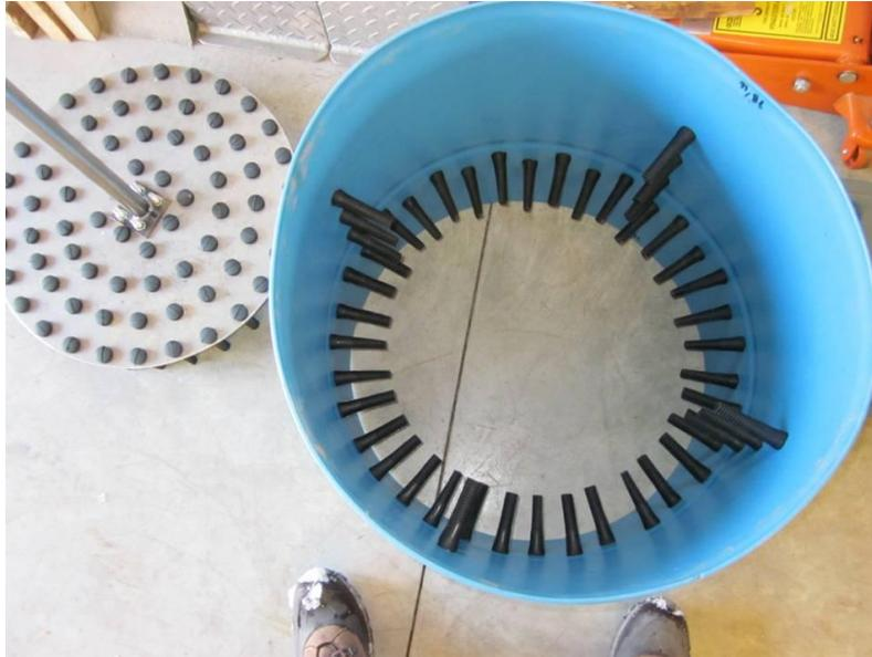
We've been working through the designs making a Whizbang plucker (google that) - we are almost there. Our design has a slight modification on the belt tensioning, which will take place with the motor mount rather than an idler pulley. It won't be pretty but it'll pluck a chicken just fine.
